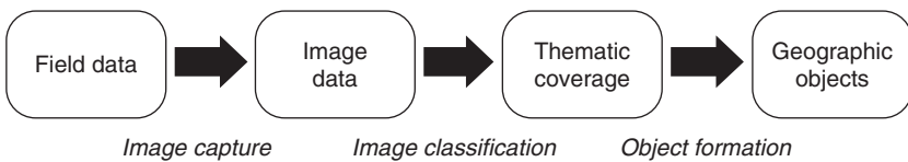
FIGURE 2.9 Continuum of abstraction from field model to object model. Continuously varying fields are quantized by the sensing device into image form, then classified and finally transformed into discrete geographic objects. (Adapted from Gahegan and Ehlers, 2000.)
